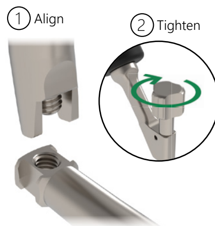
Figure 11.3 Assembly process to attach MIS Rod
