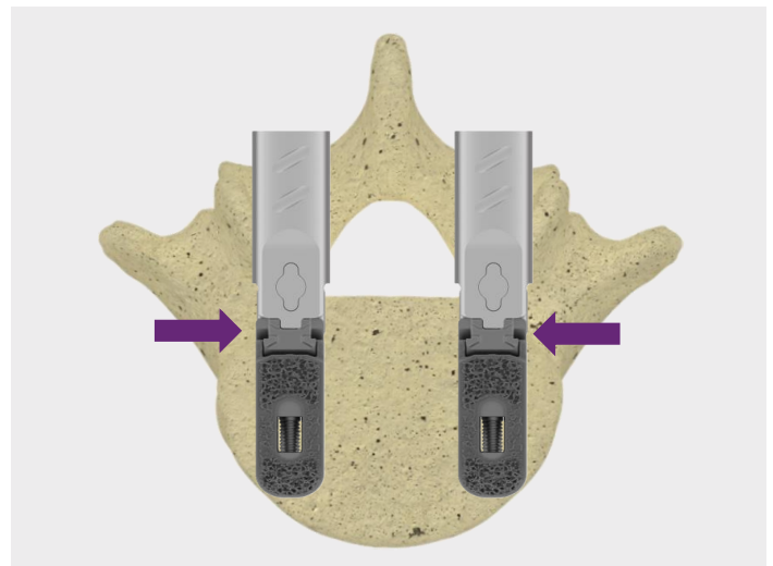
Figure 15b. The distance from the posterior scallops on the implant endplates are 2 mm from the most posterior aspect of the cage in a PLIF position.
