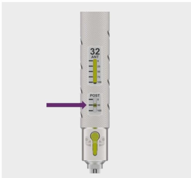
Figure 20. The posterior scale on the indicating Strike Plate may be used to assess the relative percentage of device expansion (0-100%).
