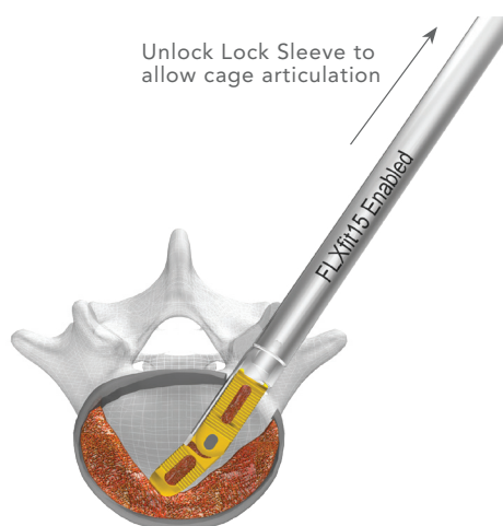
CAGE AND INSERTER ENTERING INTO DISC SPACE
