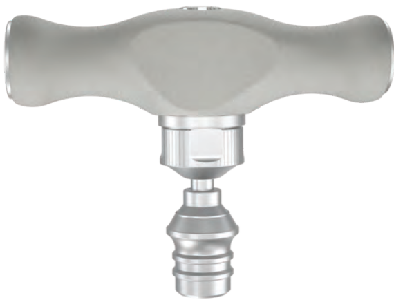
Torque-Limiting T-Handle, Ratcheting, 10Nm, 1/4" Quick-Connect 6120.0040
