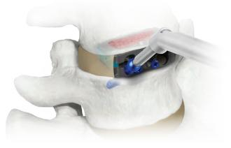
Inserting screw using Angled Screwdriver
