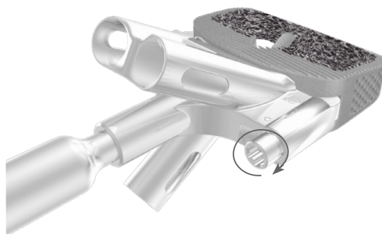
DTS GUIDE LATERAL PIN TURN CLOCKWISE TO TIGHTEN
