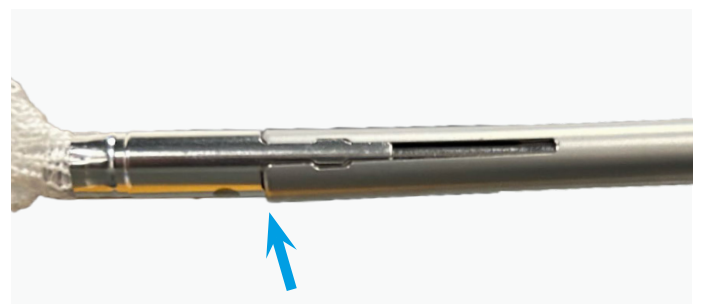
Figure 49: Image showing the Align implant loaded incorrectly, causing the distal fork to sit proud. This will not allow the implant pass through Access Portal.
