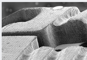
b) 0.5-micron-thick titanium layer
