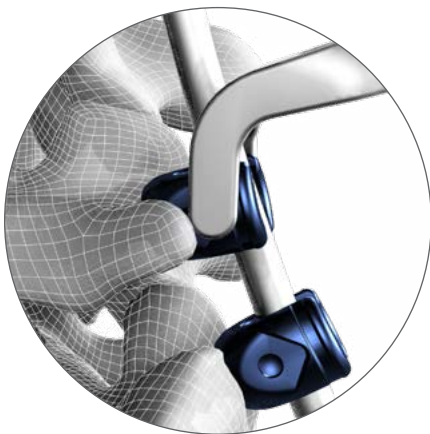
ROD ROCKER ARMS SLIDE INTO TRIANGULAR GROOVE ON SIDES OF TULIP HEAD
