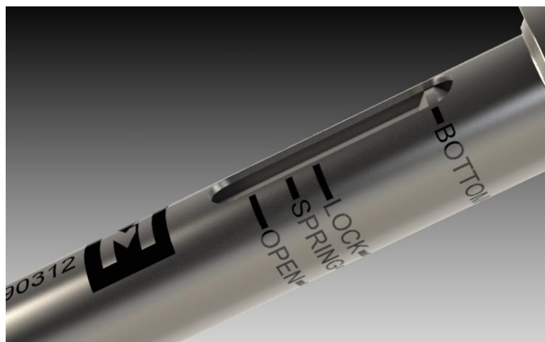
Rod reducer in the "BOTTOM" position
